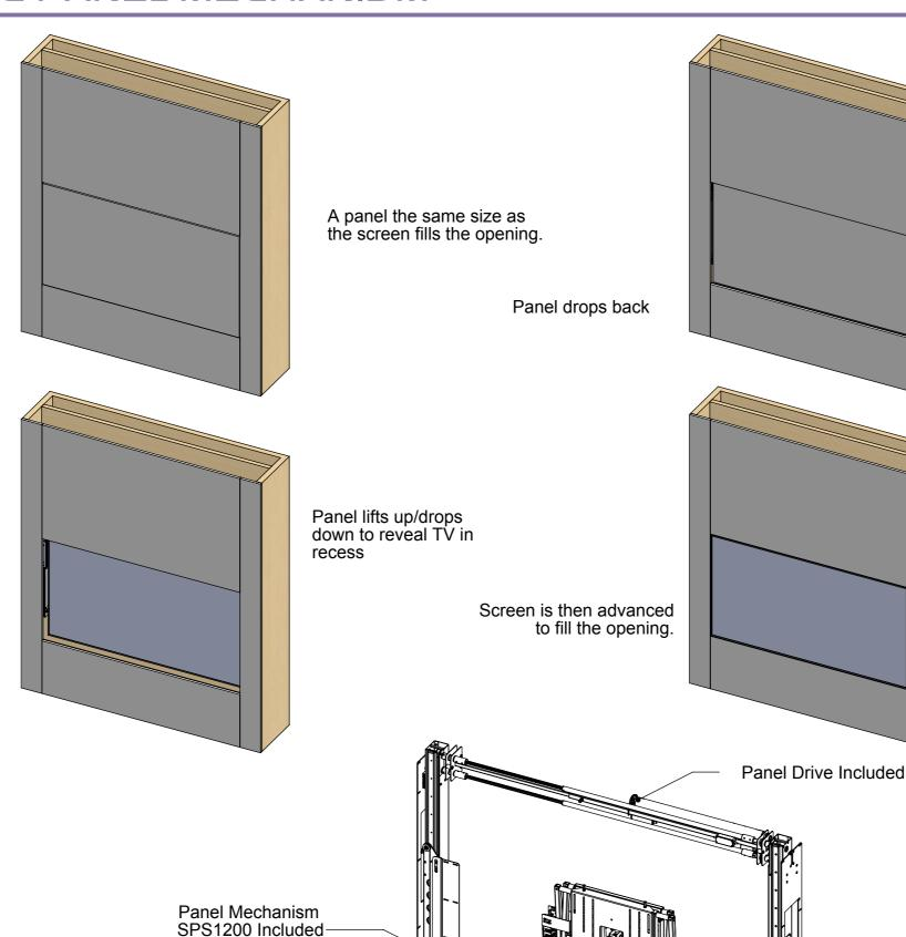
The **Panel Mechanisms** and the **Panel Drive** are all telescopic to efficiently accommodate different screen sizes.
