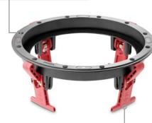
Easy Quick Install system. No tools required. System compatible with wall/ceiling from  $O^{3/16''}$  to  $1^{3/16''}$  (5 to 30mm).
