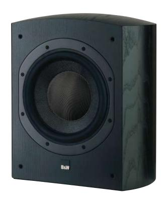
The ASW825's 12" driver features our ultra-rigid Rohacell® sandwich cone that can move prodigious amounts of air with almost perfect piston-like control. It has a 4" diameter voice coil and massive magnet assembly for high power handling without compression, which enables the subwoofer to produce true low-frequency sounds, from the subtle recreation of the acoustic of a large space to the most demanding film special effect.
