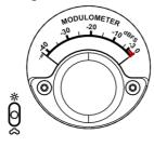
Nagra Modulometer is inherited from the second recorder developed by Nagra back in 1952, the Nagra II. The Modulometer is a typical Nagra precision instrument that displays the necessary information to perform the best possible recordings. In the case of the CLASSIC DAC, the Modulometer displays the digital input level. The 0 dB corresponds to full scale signal, meaning the maximum digital level.
