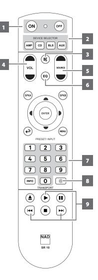
The SR 10 remote control handset handles the key functions of the C 3050. It can also control up to 4 devices. The SR 10 can operate up to a distance of 23 ft (7m). Alkaline batteries are recommended for maximum operating life. Two AA batteries must be fitted in the battery compartment at the rear of the remote control handset. When replacing batteries, check that they have been put in the right way round, as indicated on the base of the battery compartment.
