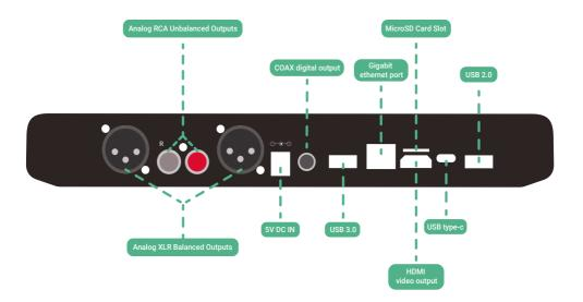
**ANALOG XLR BALANCED OUTPUTS:** XLR Output connection will allow you to run longer lengths of wire without picking up interference. If you own an amplifier with XLR inputs, this connection gives you a cleaner audio signal. Suggested connection to achieve best performances from Primo's integrated high resolution DAC.
