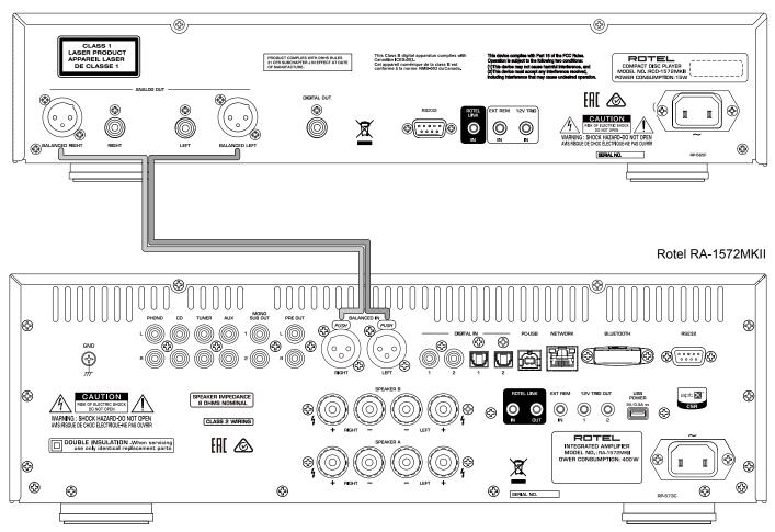
Figure 5 : Digital Output Connection
