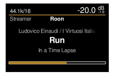
When turning the MU1 main control knob, the volume changes and the track progress bar at the bottom is temporarily replaced by a bar that indicates the current volume setting. The MU1 will send volume control data to the DSP of the LS1 via its proprietary cat5 cable. For 3<sup>rd</sup> party DACs the
