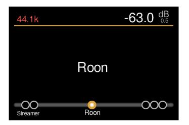
By turning the main knob (while holding it down) the different sources are selected.
