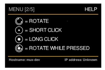
This menu explains the pictograms that are used in the MU1 for operating the main knob. At the bottom the network information is shown. When the IP address is unknown, there is no network connection and the MU1 cannot be found by the Roon control app in your tablet or smart phone.
