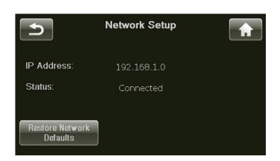
The Delta PRE includes a built-in web interface that can be used to configure the system name, Network settings or update the Delta PRE software. To access the interface, type the IP address displayed on the Network Setup page in the URL line of your browser (e.g. 192.168.1.0) and hit return. Alternately if you are using Safari on the Mac, you can "Show All Bookmarks" (See: Bookmarks menu) and click on Bonjour and double click on your Delta PRE device listed in the Webpage's folder.
