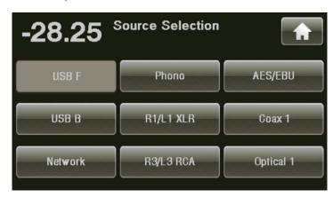
Touch any **source** button on the touchscreen to select it as the current source. The selected source button is shaded. If the source you want to choose is not on this screen (and you have more than nine source buttons enabled), press the button for the next page of sources. Or, press the previous page.
