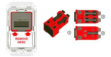
An additional fuse mark on the switch indicates the fuses holders behind the switch. The red frame shows the outline of the removable unit.
