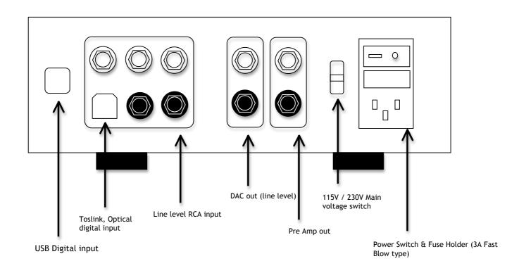
Avoid static shocks to the inputs or outputs. Before connecting or removing a cable, touch any grounded surface, such as the chassis of a component that is plugged into an AC socket. Inputs and outputs can be safely connected to the Burson Conductor when its AC power is switched off.
