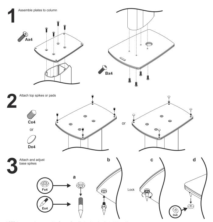
NOTE: In case you have a sensitive floor surface (like hardwood or tiles) which could be damaged by the spikes, please use the spike plates included in the kit (G)
