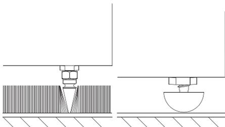
The 803 Diamond and 804 Diamond can be fitted with either rubber or spike feet – both are supplied in the accessory pack. We would recommend that the spike feet are used whenever possible. The spike feet are designed to pierce carpet and rest on the floor beneath, both to protect the carpet from indentation and to provide the speaker with a solid foundation.
